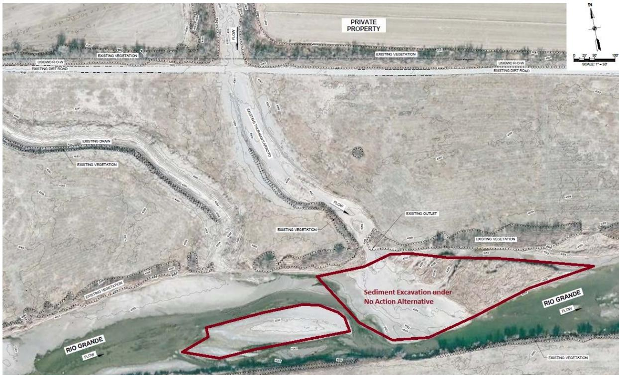
**Figure 2-2. Area of routine sediment excavation at Thurman II under Alternative B - No Action (modified from USIBWC 2017b)**
