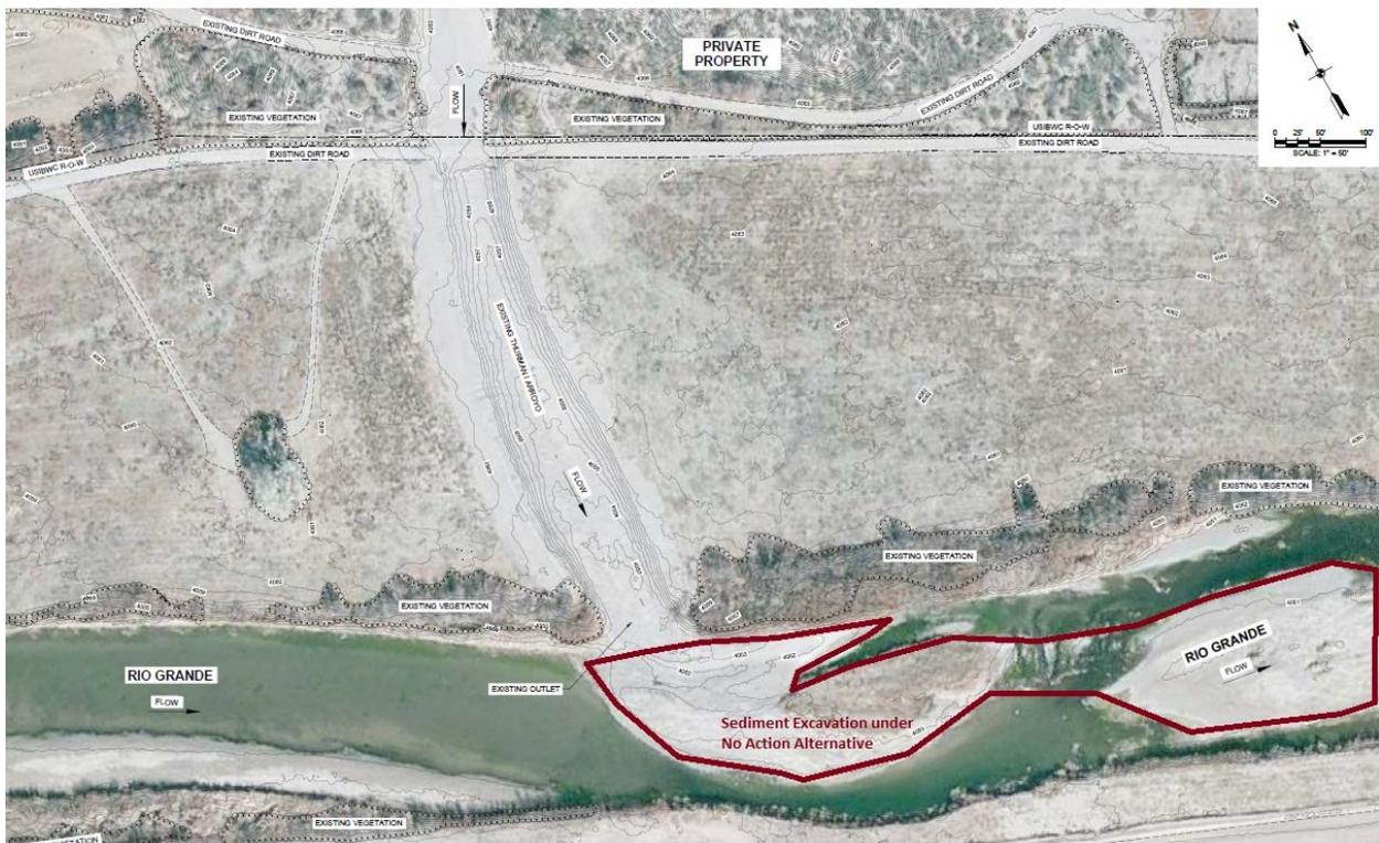
**Figure 2-1. Area of routine sediment excavation at Thurman I under Alternative B - No Action (modified from USIBWC 2017b)**
