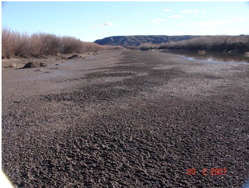
Figure A.19. Close up view of the bar materials at sample S-3. The D_{50} of the bar materials is 4 mm (S-3).
