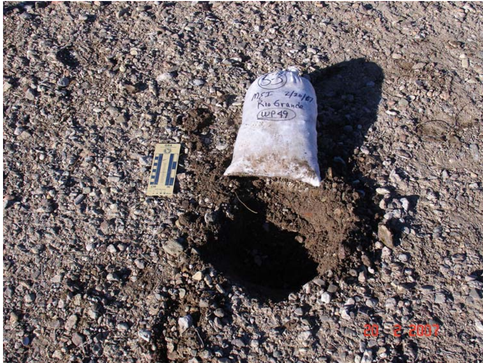
Figure A.19. Close up view of the bar materials at sample S-3. The D_{50} of the bar materials is 4 mm (S-3).
