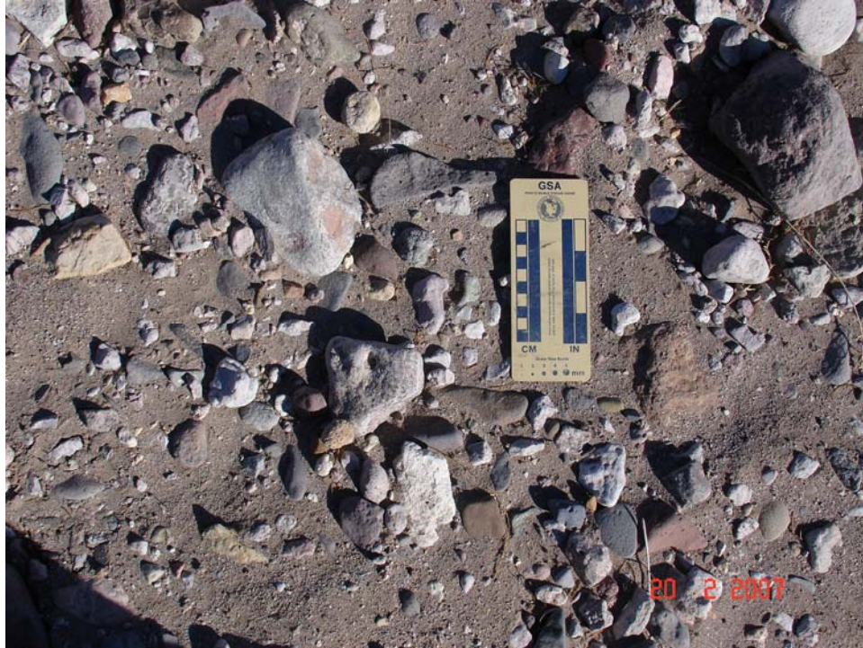
Figure A.17. Close up view of un-reworked sediments on the Tierra Blanca fan that had a D_{50} of 16 mm (S-2).
