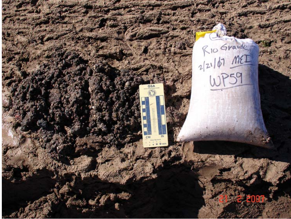
Figure A.25. Close up view of the subaqueous sample that was collected upstream of the Hatch Siphon (S-4#2). The D_{50} of the bed materials is 2.2 mm.
