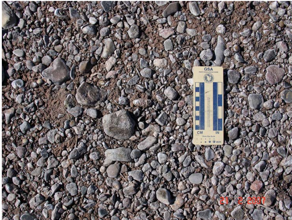
Figure A.27. Close up view of the surface sediments on the gravel bar downstream of Salem Bridge. The D_{50} of the bar materials is 0.34 mm (S-5).
