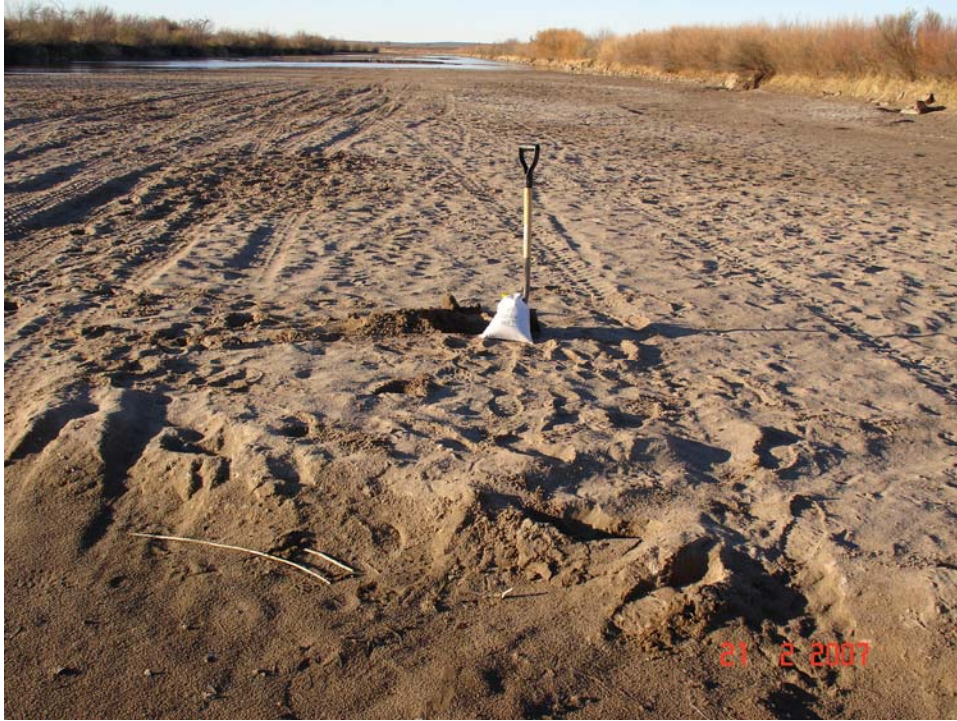
Figure A.29. View upstream of the bed of the Rio Grande at Mile 54 Cut where sample S-9 was collected. The D_{50} of the bar materials is 0.4 mm.
