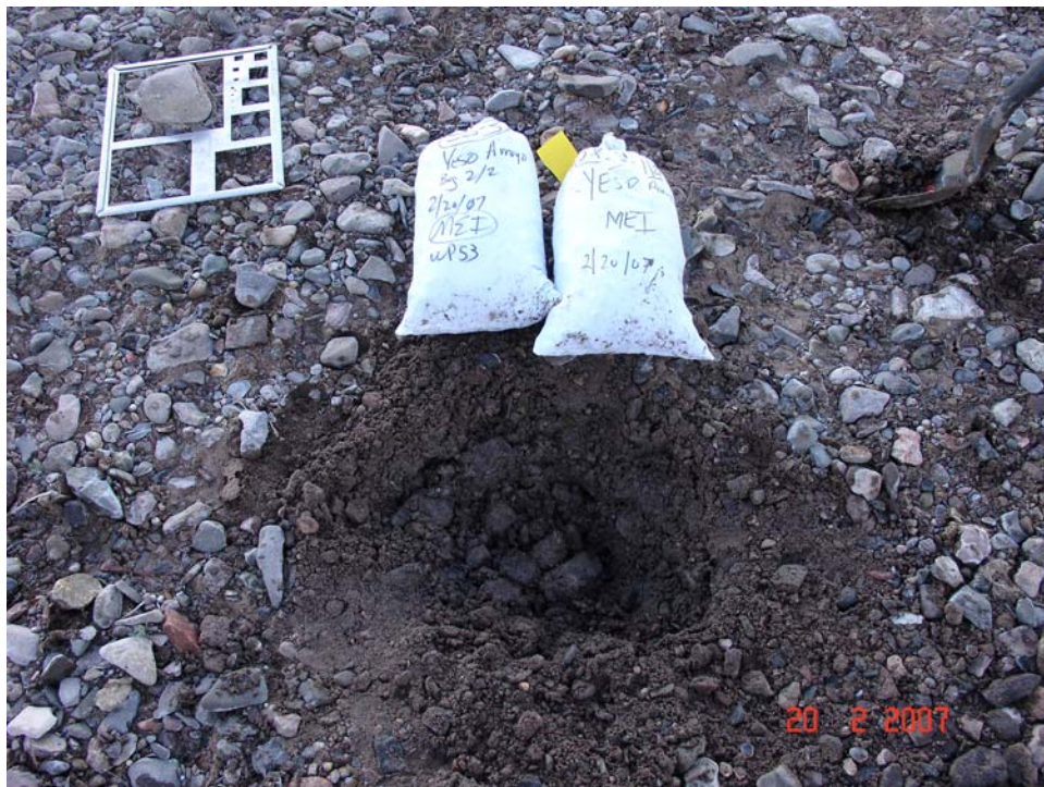
Figure A.24. Close up view of the subsurface sediments at the gravel bar downstream of Yeso Arroyo. The D_{50} of the subsurface materials is 21 mm (SS-2).
