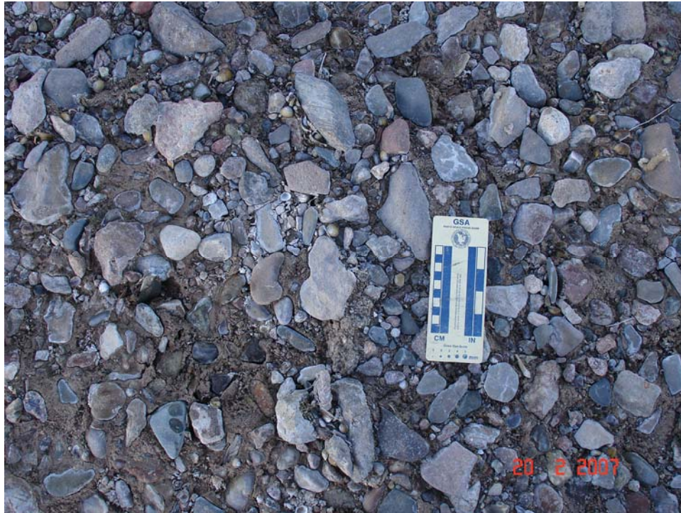
Figure A.23. Close up view of the gravel bar surface sediments downstream of Yeso Arroyo that were sampled with a pebble count (WC-3). The D_{50} of the surface materials is 47 mm (S-3).
