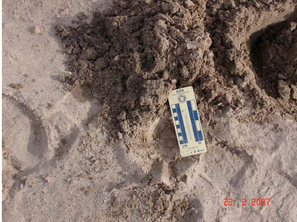
Figure A.33. Close up view of sample S-11 on the surface of an alternate bar located 2.1 miles downstream of the Mesilla Bridge. The D_{50} of the bar materials is 0.29 mm.
