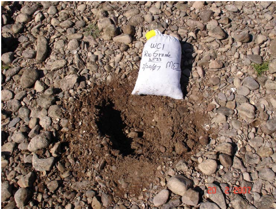
Figure A.12. Close up view of bar surface and subsurface sediments where WC 1 and SS-1 ( D_{50} = 15.6 mm) were collected.
