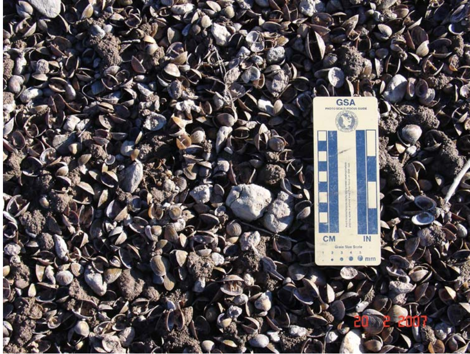
Figure A.21. Close up view of bar surface covered with freshwater mussel shells at the Sibley Point Bar site where sample S-4 was collected ( D_{50} = 0.14 mm).
