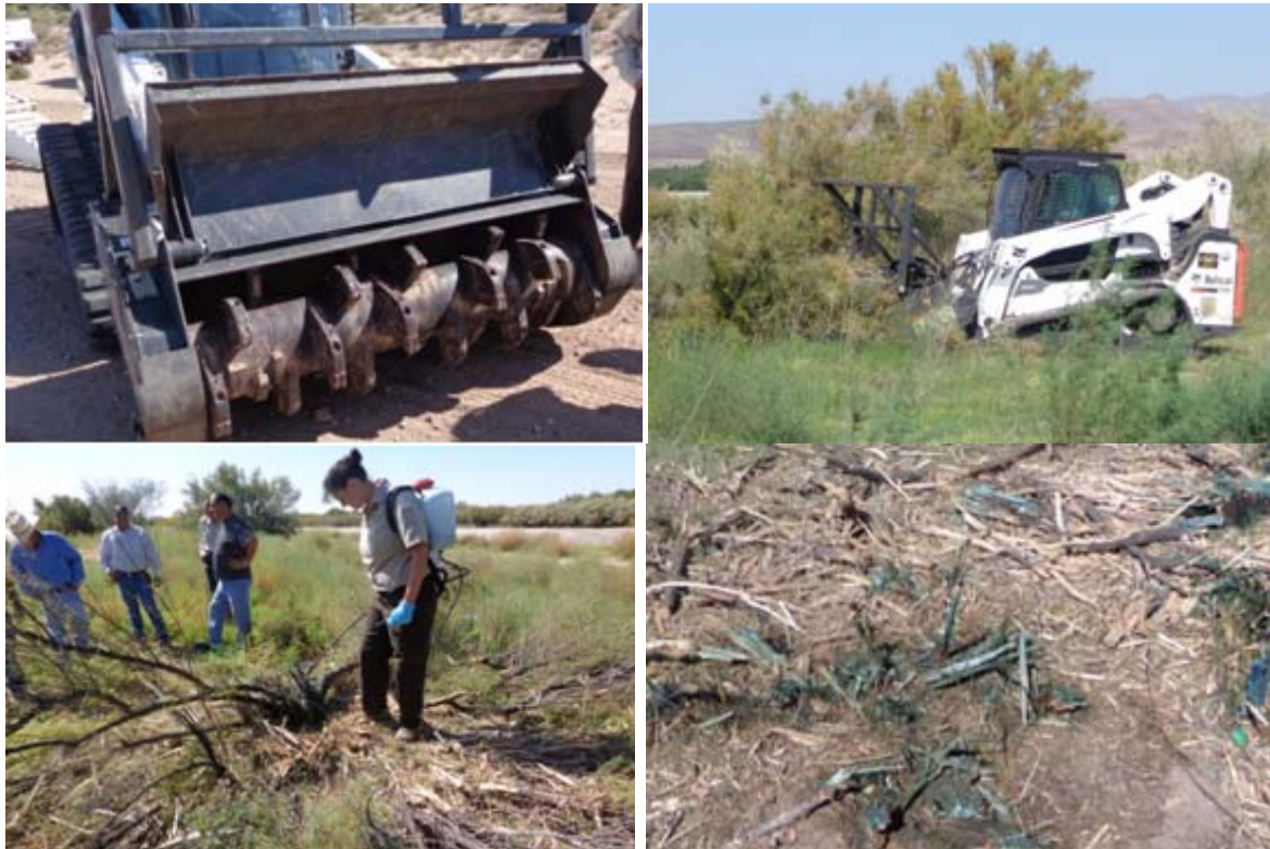
Figure 2-7. Mechanical and Herbicide Treatment method. A) Top left - example attachment on skid steer loader. B) Top right - equipment mulching large saltcedar. C) Bottom left - herbicide application on cut saltcedar stems. D) Bottom right - after herbicide.
