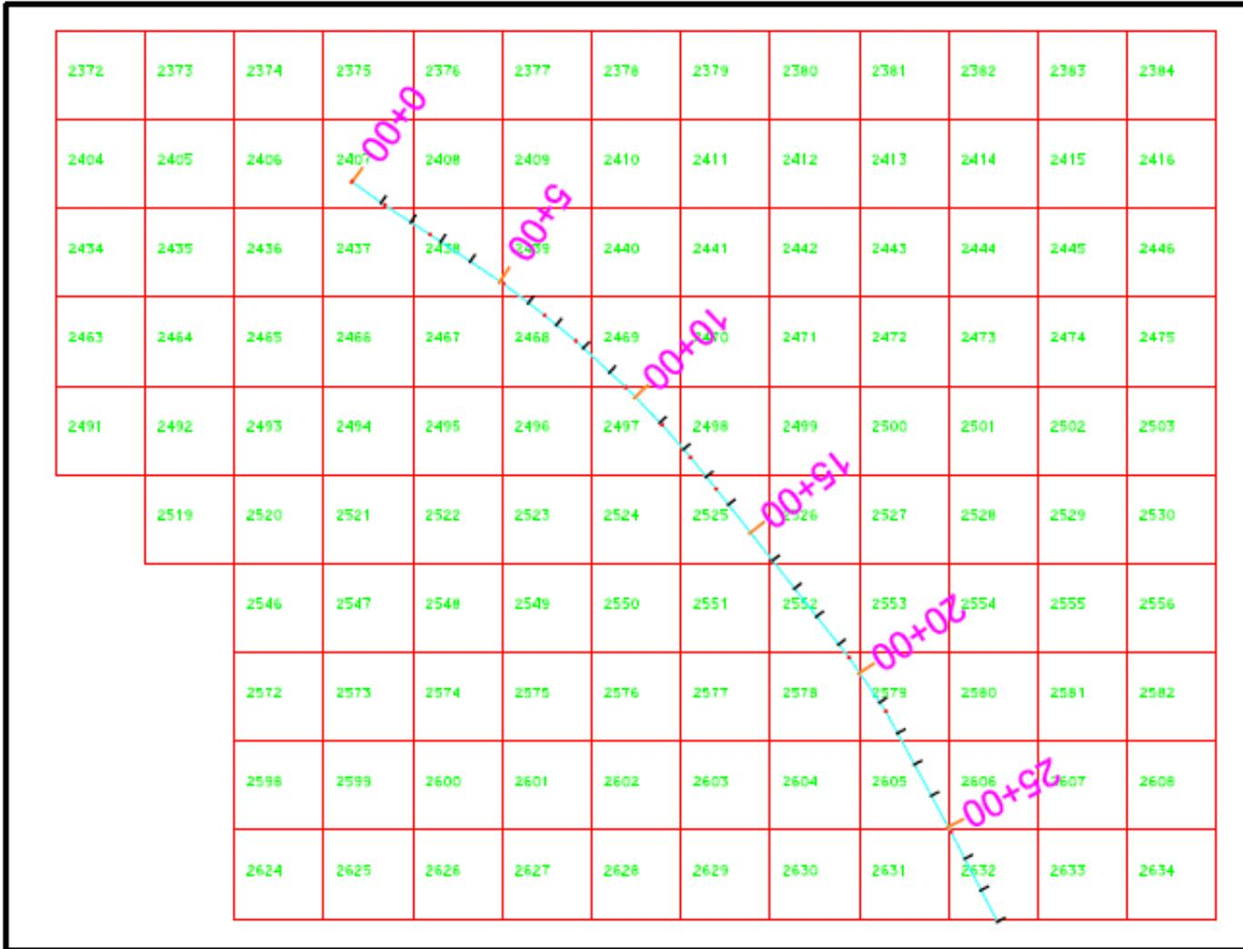
Figure 10. Typical Levee Alignment with Respect to the FLO-2D Grid System
