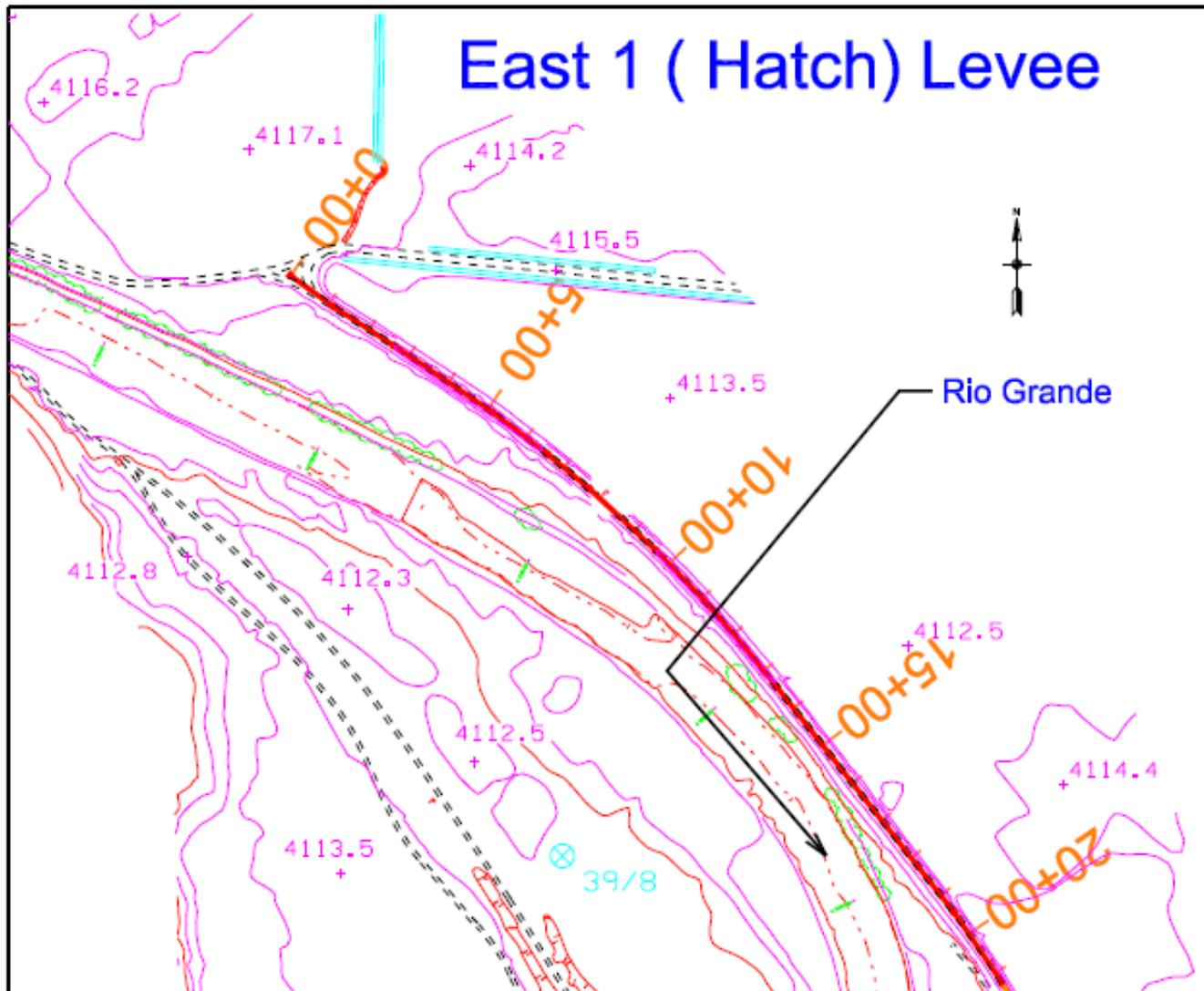
Figure 9. Typical Horizontal Levee Centerline Alignment Using the 2 ft Contour Mapping
