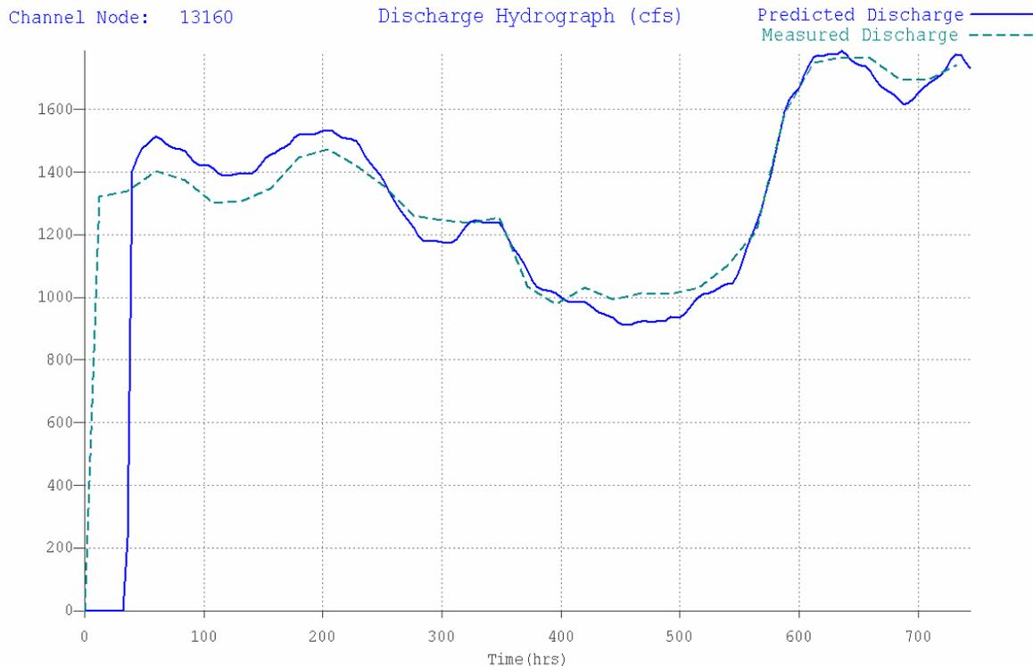
Figure 12. 2004 Haydon Gage Data vs. FLO-2D Predicted Hydrograph
