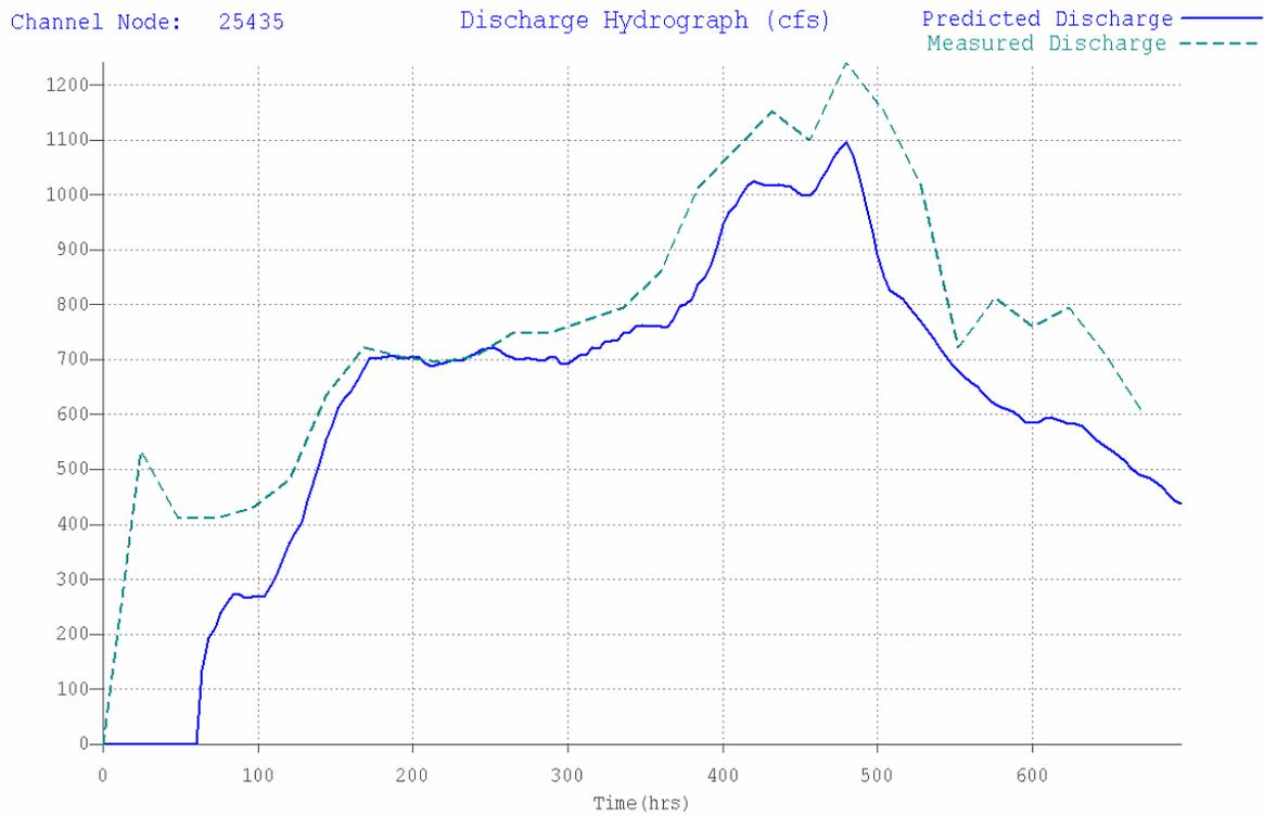
Figure 21. 1998 Mesilla Gage vs. FLO-2D Predicted Hydrograph
