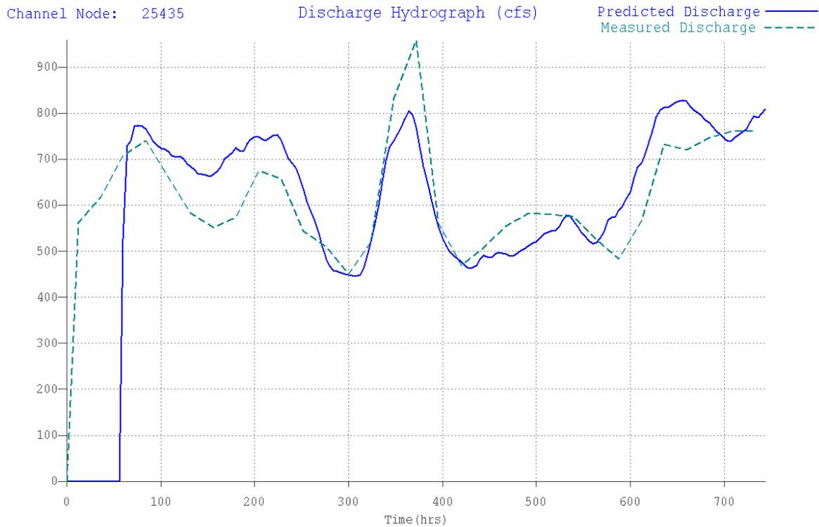
Figure 14. 2004 Mesilla Gage vs. FLO-2D Predicted Hydrograph
