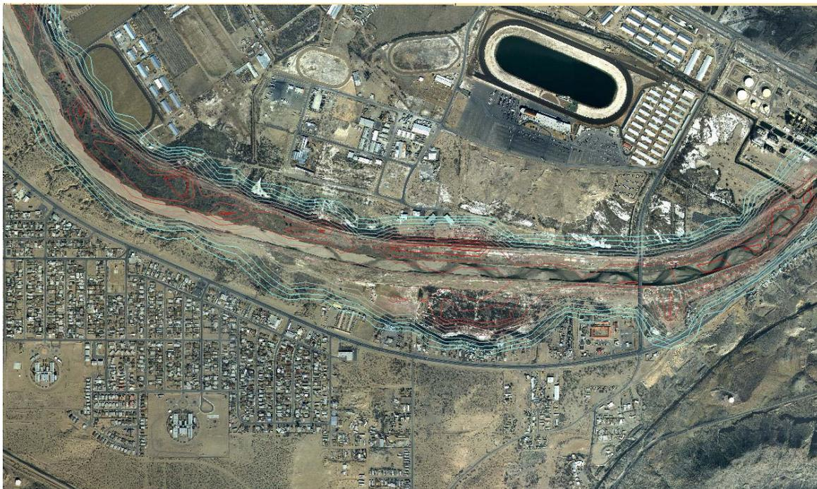
Figure 25. Example of the Area of Inundation for the 100-yr 24-hr Storm,
