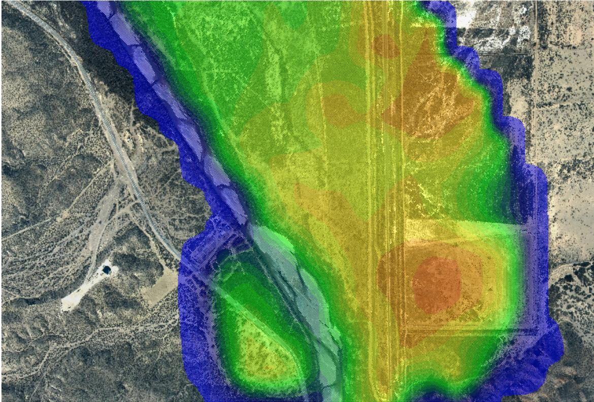
Figure 24. Example of the Area of Inundation for the 100-yr 24-hr Storm
