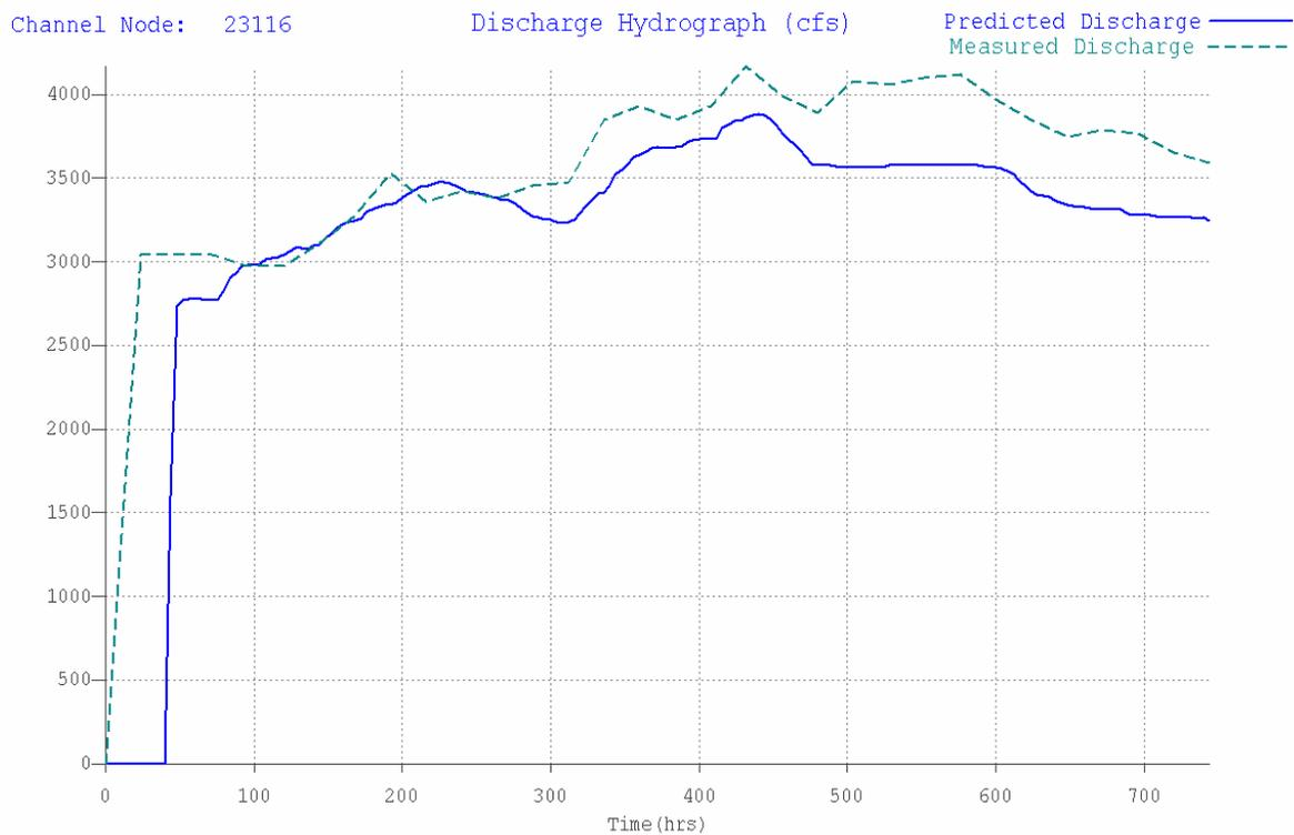
Figure 17. 1995 Picacho Gage vs. FLO-2D Predicted Hydrograph
