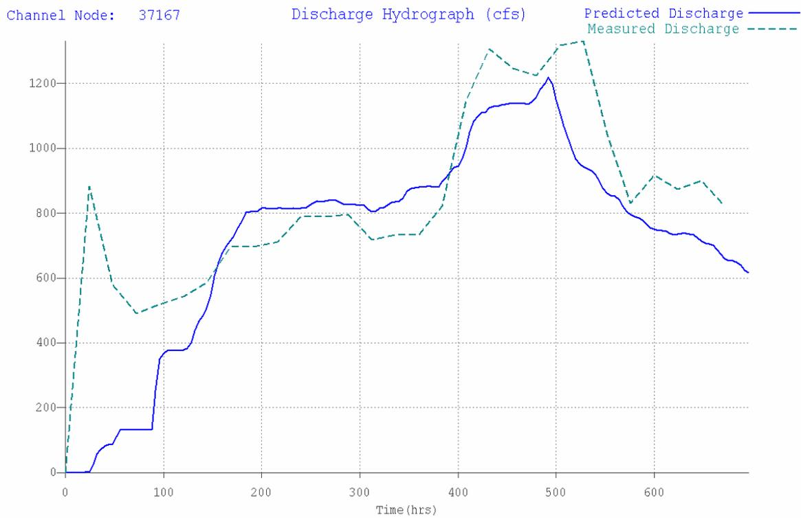
Figure 22. 1998 Canutillo Gage vs. FLO-2D Predicted Hydrograph
