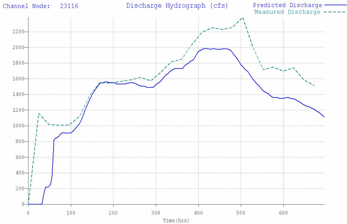
Figure 20. 1998 Picacho Gage vs. FLO-2D Predicted Hydrograph
