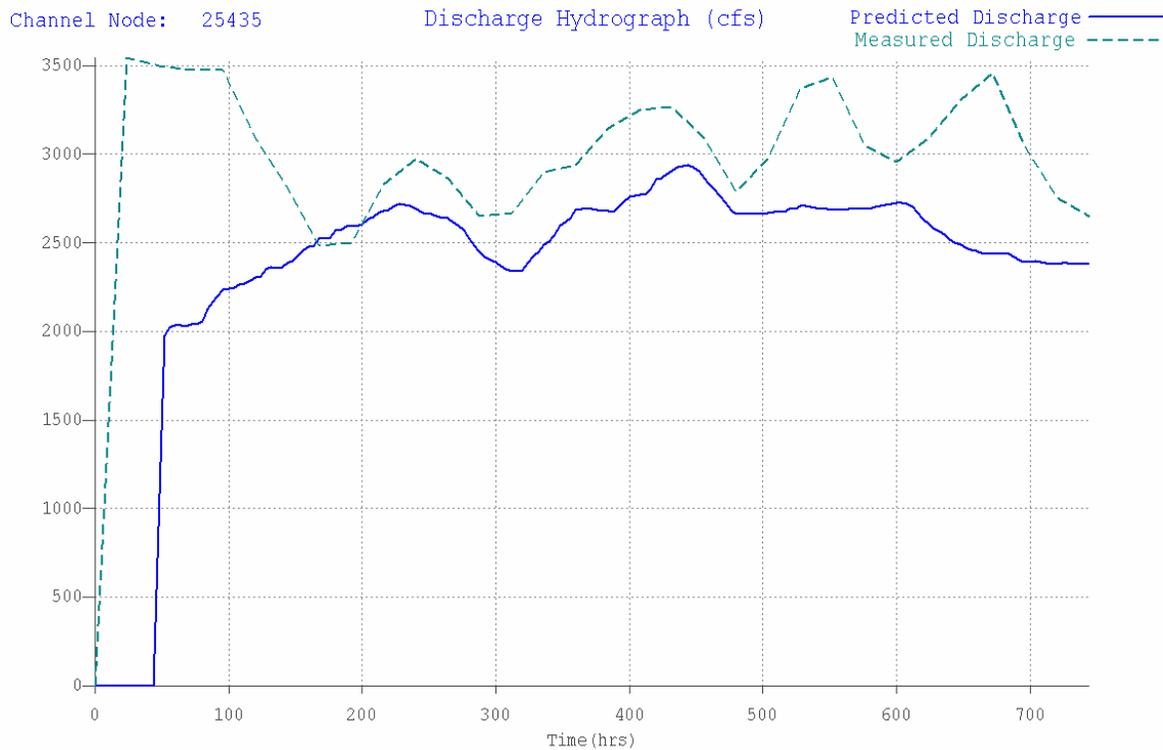
Figure 18. 1995 Mesilla Gage vs. FLO-2D Predicted Hydrograph
