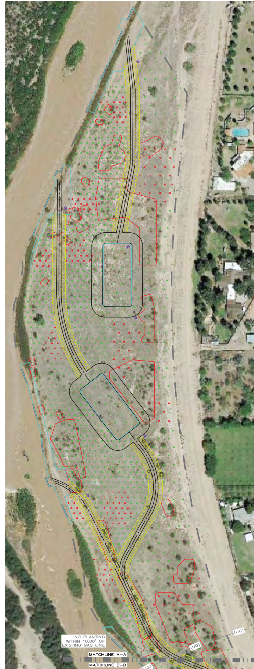
SUGGESTED COYOTE WILLOW POLES PLANT PATTERNS NOT TO SCALE
