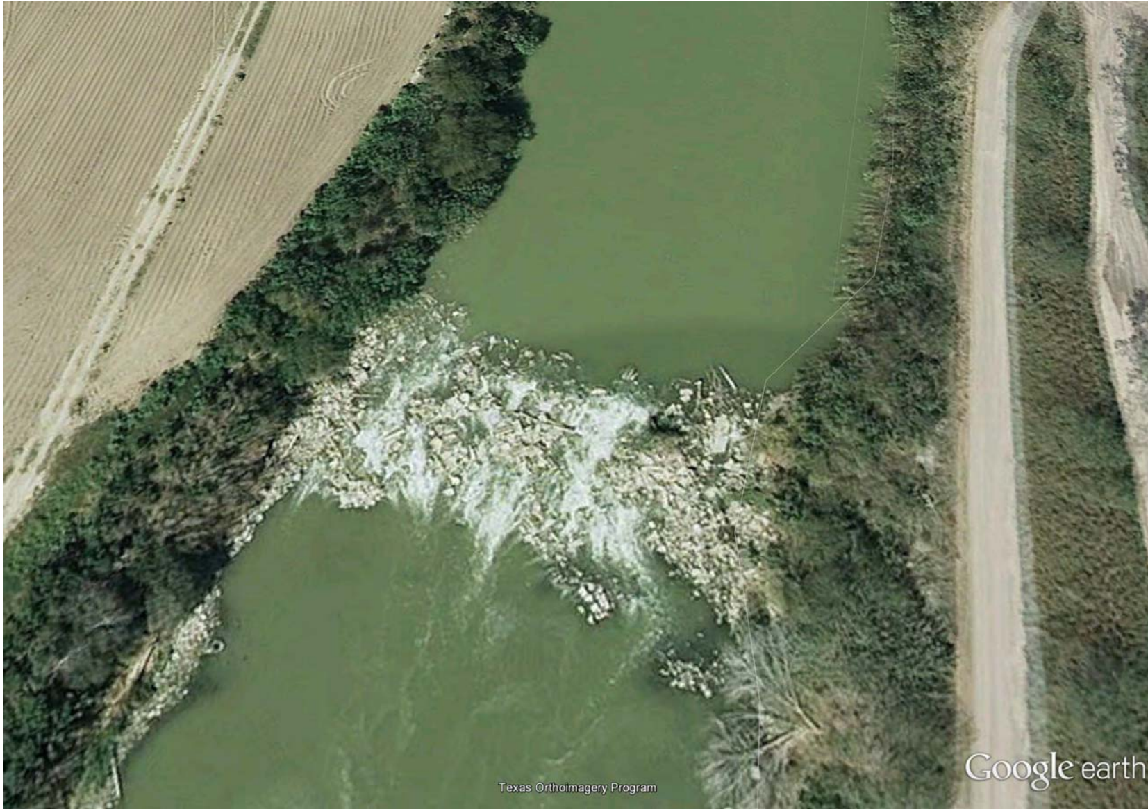
Figure 5.13. Google image of the rock boulders and cobbles that were used to build the grade control structure upstream of the Brownsville gage.
