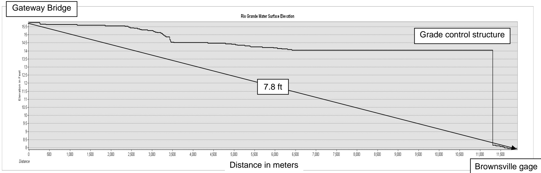
Figure 5.11. Change in water surface elevation between the Gateway International Bridge and the Brownsville gage. The presence of a grade control structure occurs 213 m (750 ft) upstream of the gage. Water surface data presented above derived from the 2011 LiDAR data of the Brownsville area.
