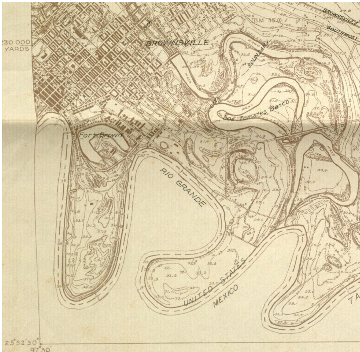
Figure 3.4. Portion of the USGS East Brownsville topographic map showing detailed 1-ft contour interval and spot elevations in feet MSL (mean sea level) (USGS 1930). Note the width of the river channel through the bend way, the presence of Gateway International Bridge, crossing of the water surface elevation contour of 16 ft MSL at downstream edge of the study area, the detailed contour information for the abandoned oxbow (banco), the levee alignment, and spot elevations shown on nearby oxbows.
