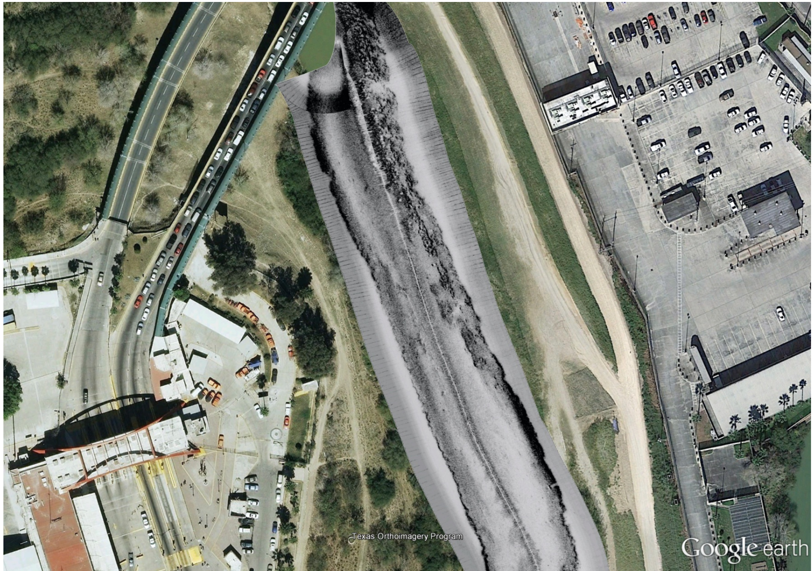
Figure 4.18. Side scan sonar image overlain on 2014 Google image showing the channel of the Rio Grande through the study area. Close-up view presented in Figure 4.19 with prominent features noted.
