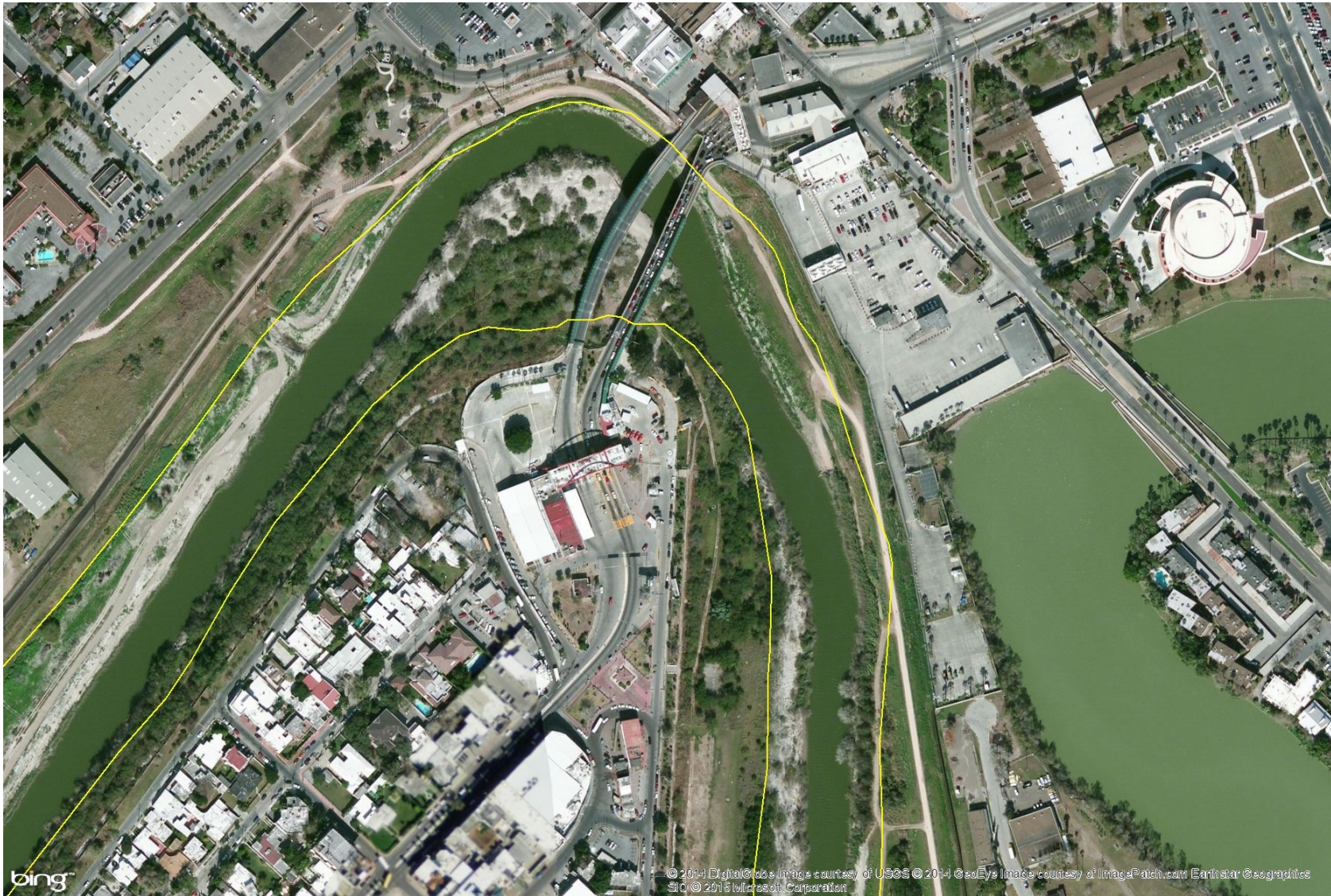
Figure 3.11. 2013 Bing image with 1930 Rio Grande channel limits shown by yellow lines. Edge of the 1930 river channel corresponds to approximate toe of current levee. Gateway International Bridge shown is the second bridge at this location.
