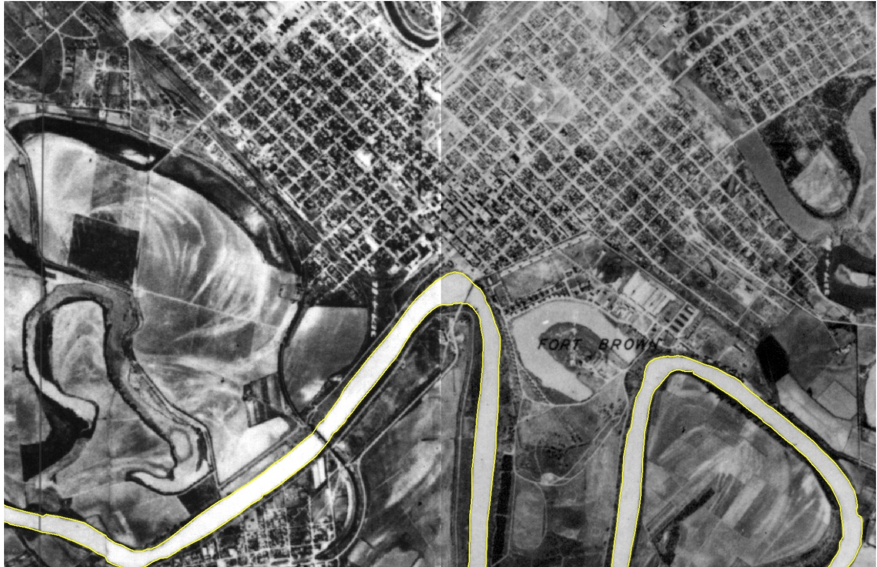
Figure 3.10. East and West Brownsville 1930 Tobin Photographs with channel limits of Rio Grande outlined in yellow.
