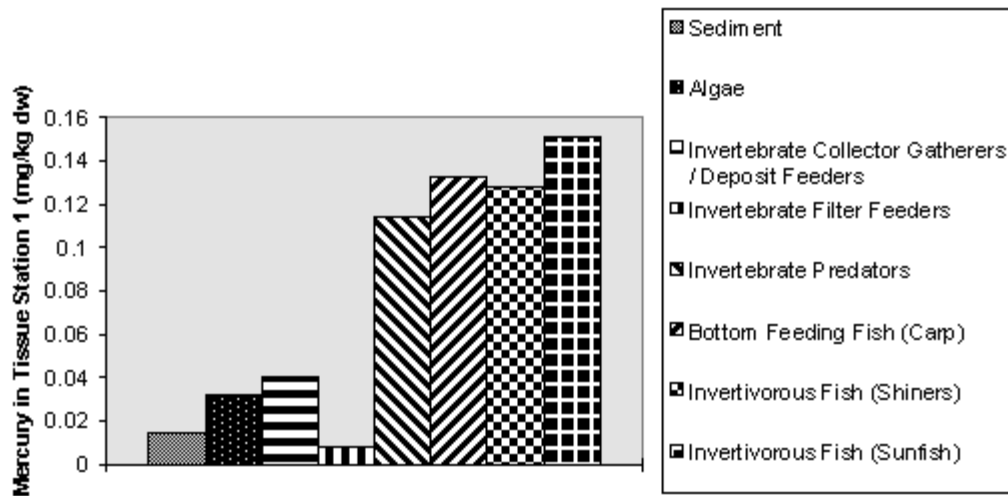
Figure 11. Summary of Mercury Concentrations in Tissue of Different Trophic Levels for Samples Collected at Station 1 During Phase III.
