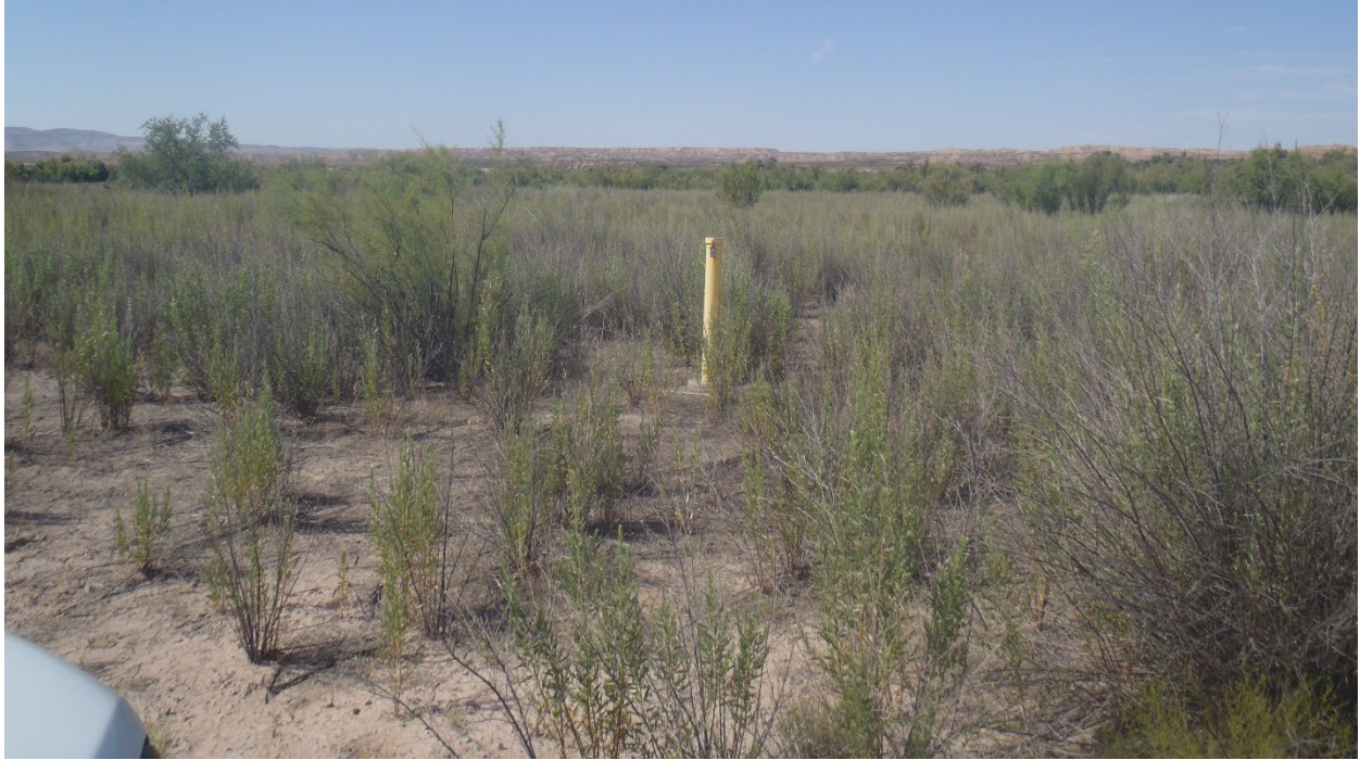
This was the well CCA-MW-1 that had the additional sonde. Unfortunately, it was not retrievable, and the well was obstructed so we couldn't get any reading on it.
