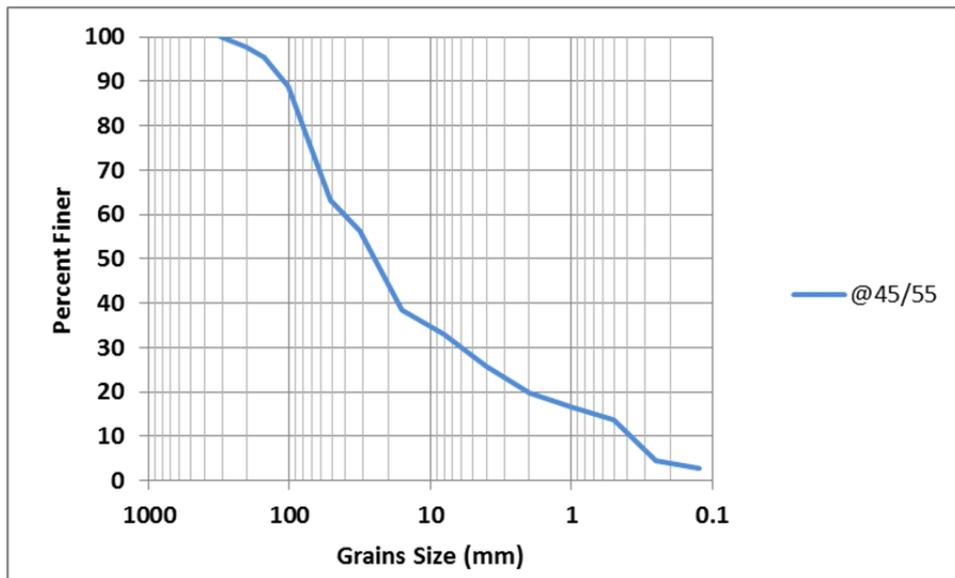
Figure A-11. Grain Size Curve after Merging the Bulk Sample and Pebble Count Data Collected from Deposits in Problem Area 2 Using the 45/55 Ratio
