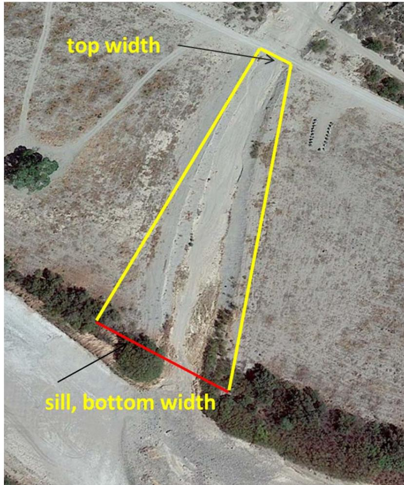
Figure A-18. Map View of Basin-Based Trap and Geometric Parameters (Sill, Top and Bottom Widths)
