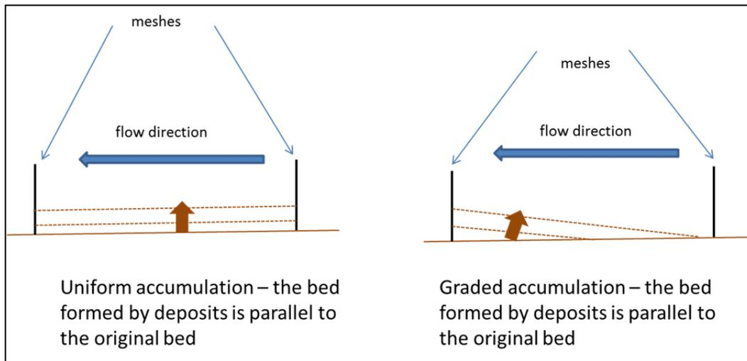
Figure A-15. Uniform and Sloped Filling Patterns.
