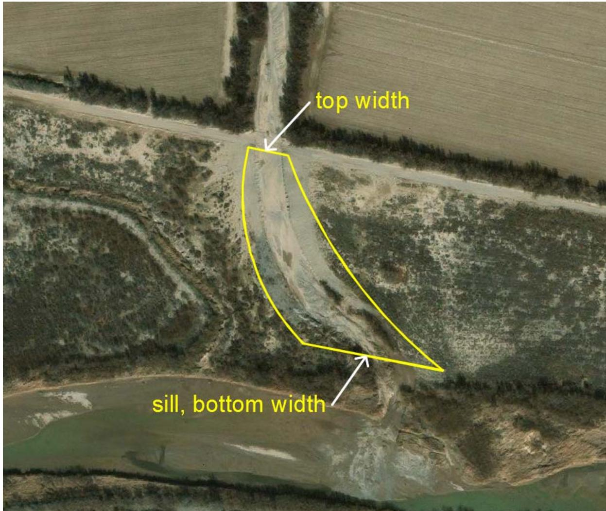
**Figure A-20. Alignment for Thurman II Basin-Based Trap**
