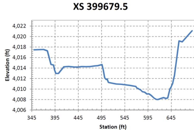
Figure B.1. Rio Grande Cross-Sections near Rio Grande AT - Hayners Bridge Near Rincon River Gage.
