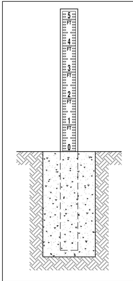
**Figure C-2. Sediment Depth Gauge Detail**
