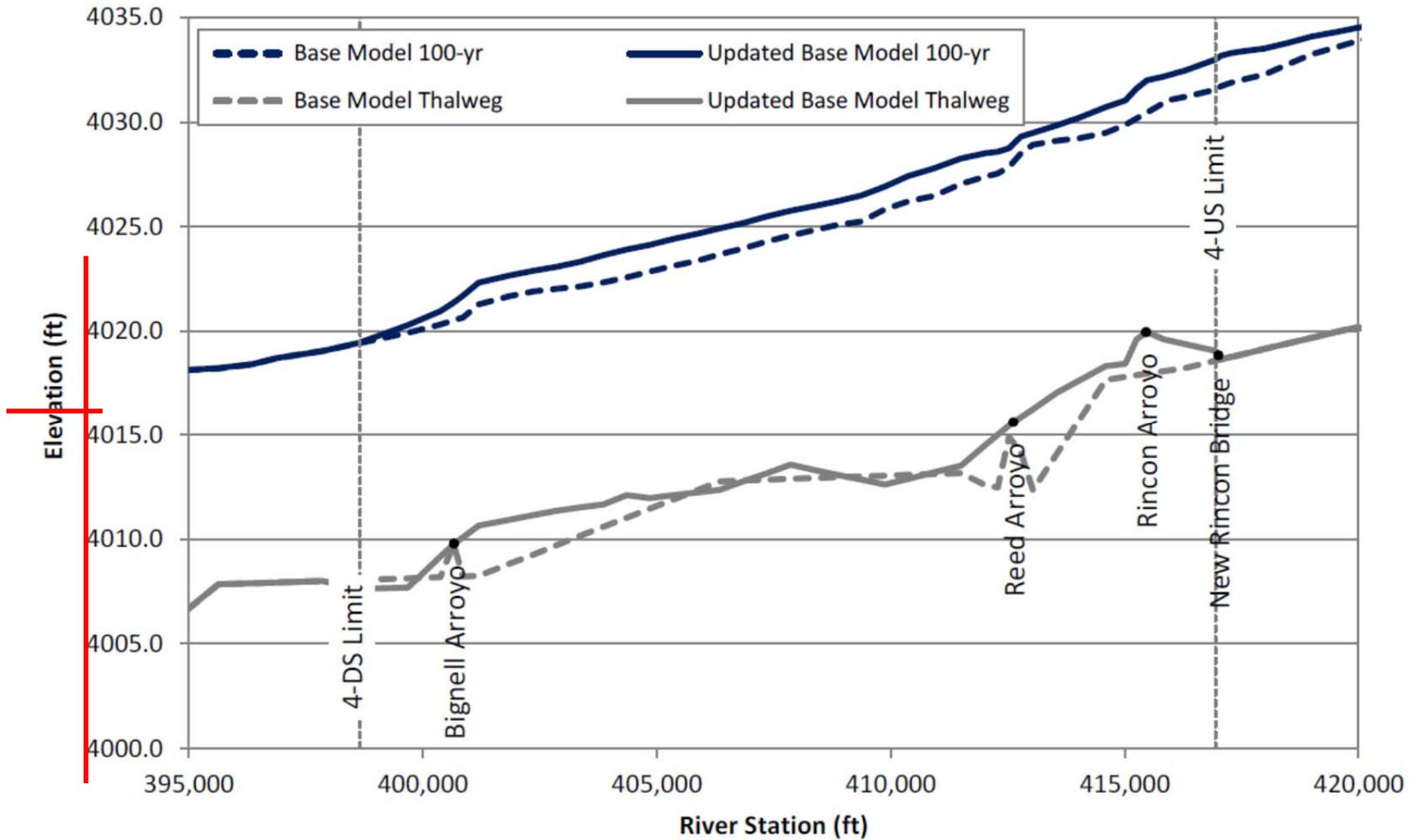
Figure B.4. Predicted water surface profiles from STA 3950+00 to 4200+00
