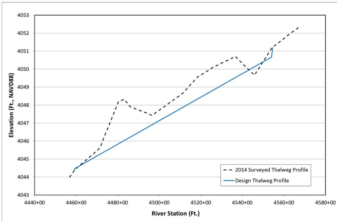
**Figure 9-1. Pre-Sediment Removal Thalweg vs. Post-Sediment Removal Thalweg**
