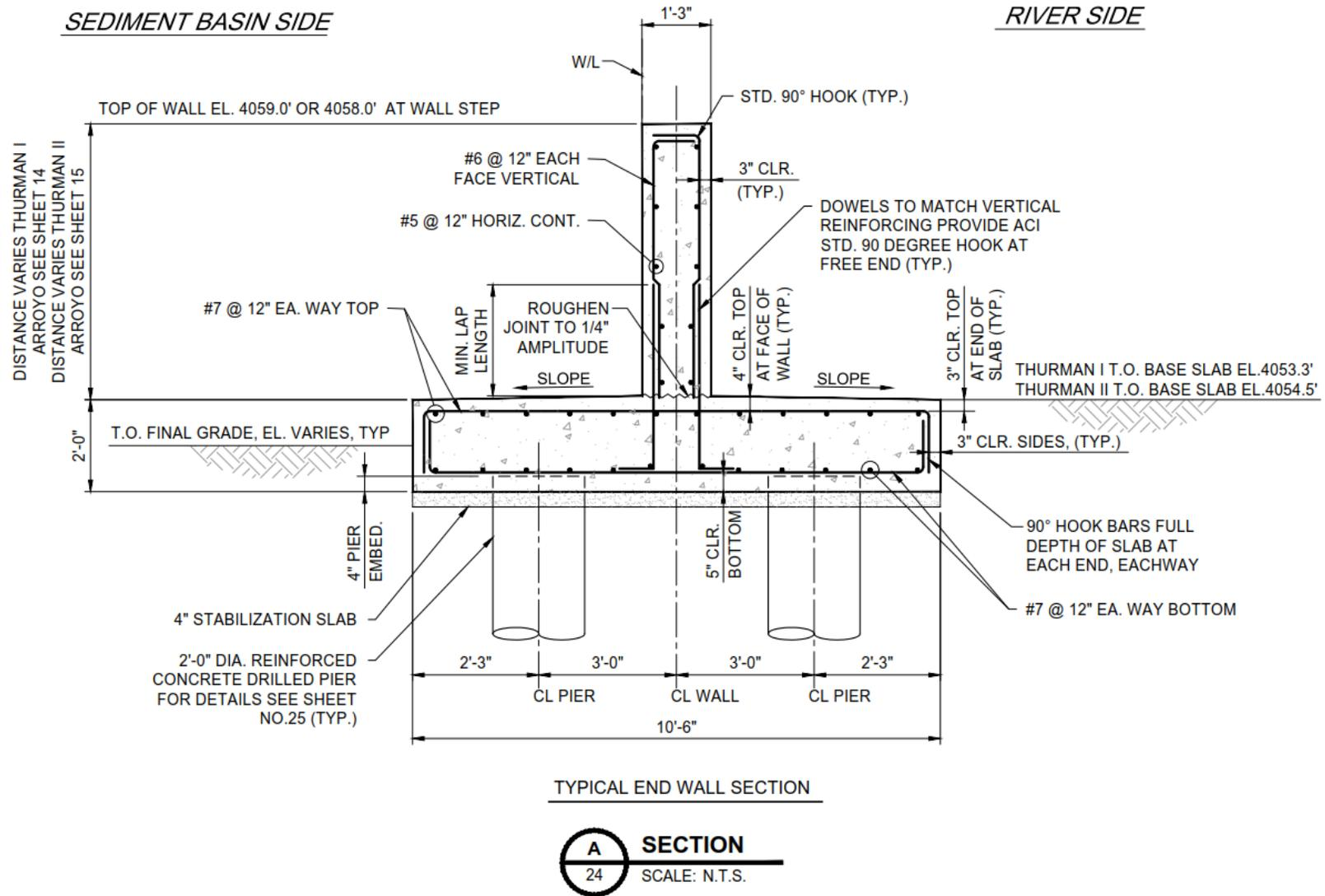
Figure 7-1. Proposed Pier-Supported Floodwall
