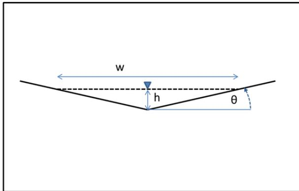
**Figure B-2. Approach for Relating Flow Width  $w$  to Flow Height  $h$**
