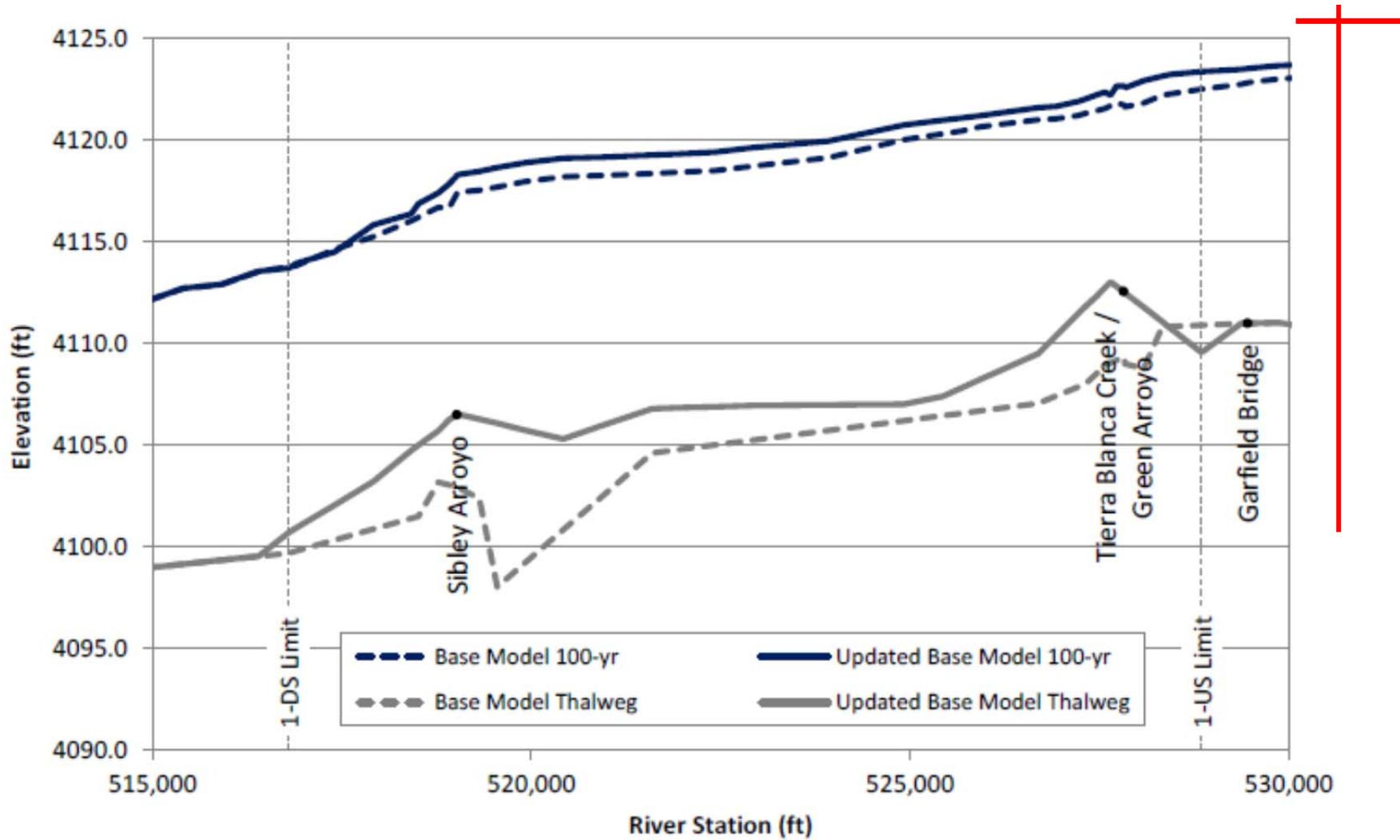
Figure B.7. Predicted water surface profiles from STA 5150+00 to 5300+00
