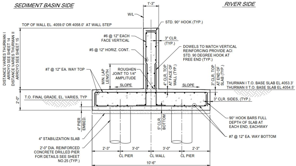
**Graphic 6-1. Drawing of End Wall for Sediment Basin.**
