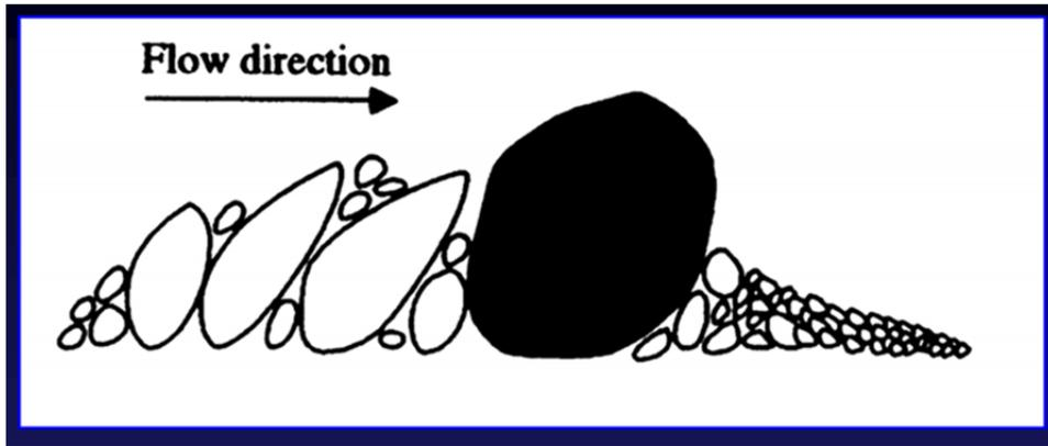
Figure A-16. Schematic Showing Hiding and Exposure of Variable-Sized Grains
