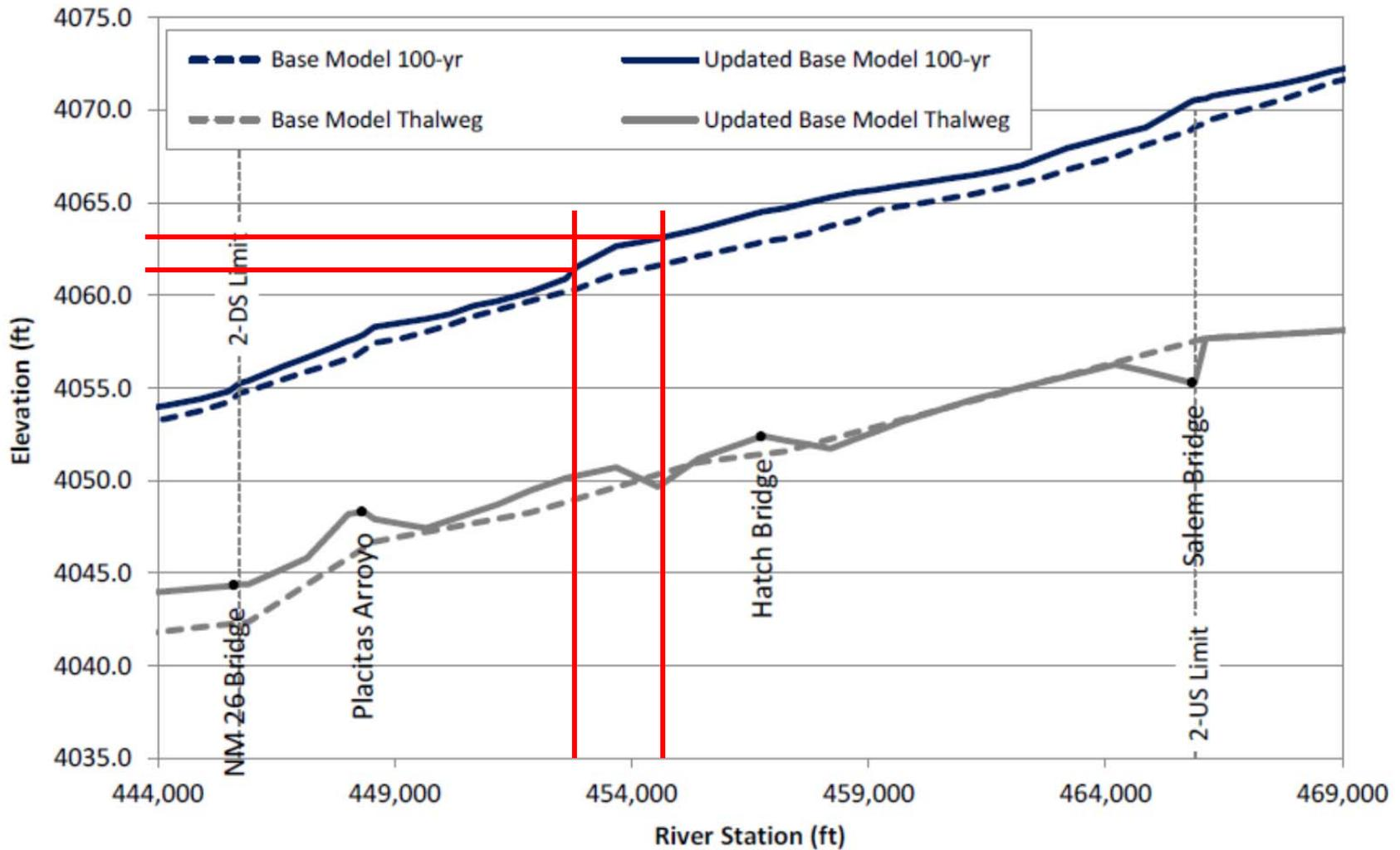
Figure B.6. Predicted water surface profiles from STA 4440+00 to 4690+00
