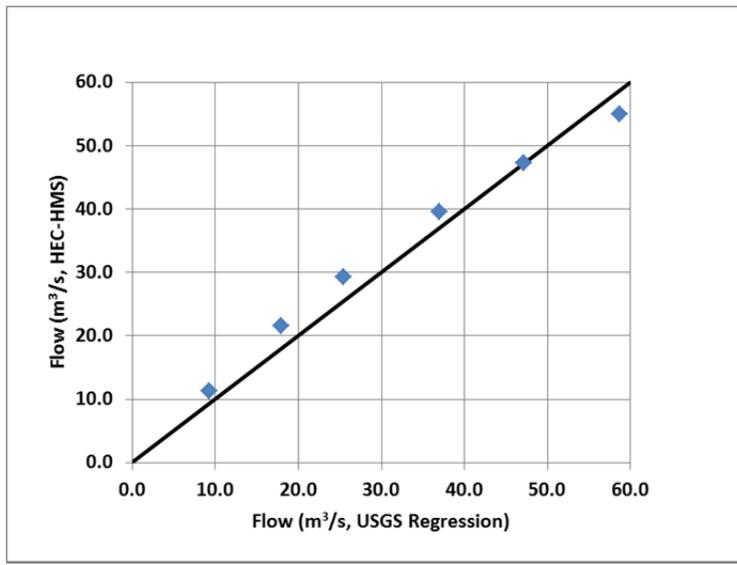
**Figure A-8. Comparison of USGS Regression-Based Discharges and Results of Return Period Analysis of Model Output for Thurman I Arroyo**
