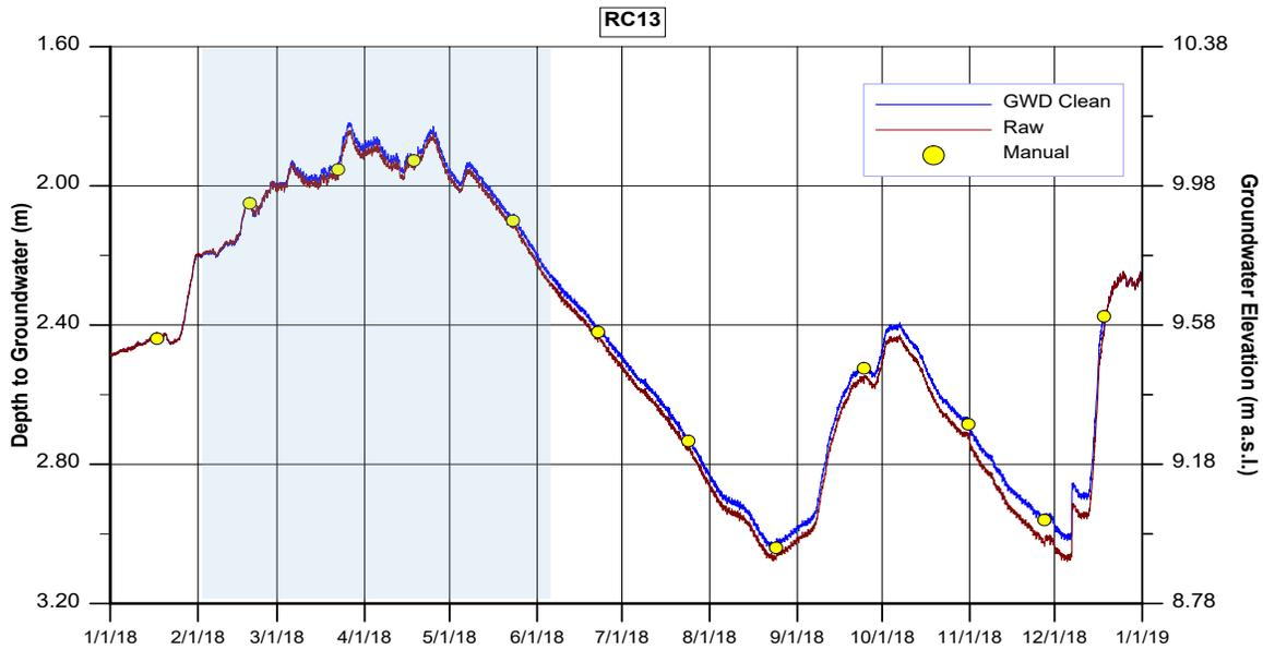
**Figure 2-6.** Depth to groundwater in piezometer RC13 (Laguna Grande). Manual=Manual measurement, Raw=Continuous registered data from the pressure transducer, GWD Clean=Continuous data corrected. Blue shaded area indicates irrigation season.
