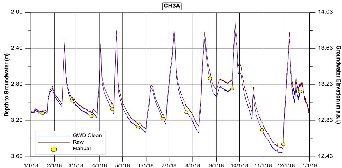
**Figure 2-5.** Depth to groundwater in piezometer CH3A (Chaussé). Manual=Manual measurement, Raw=Continuous registered data from the pressure transducer, GWD Clean= Continuous data corrected. From UABC and ETS 2019.
