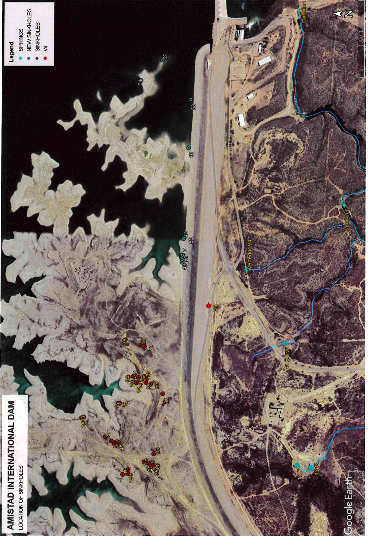
EXHIBIT II.A. Location of sinkholes
