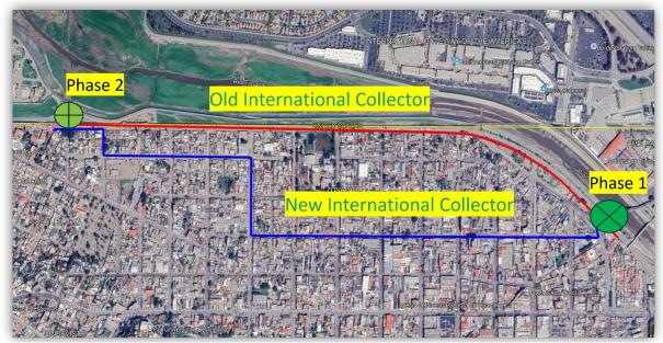
Phase 1: complete the installation of the 1.6-mile new International Collector. Phase 2: rehabilitate the section of the pipeline between Mexican junction box and pump station PB-1, which leads to Junction Box 1 at the South Bay International Wastewater Treatment Plant and install gate valves for control of flow sent to the plant.
